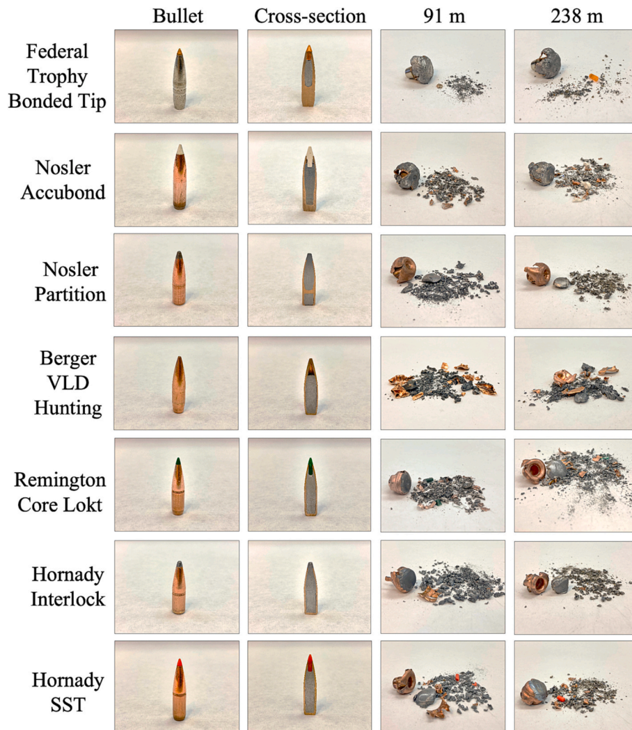
Fig. 4. The first two columns show the lead-based bullets and their cross-sections. The second two columns show their expansion and fragmentation at 91 m and 238 m. after being fired into water containers. On average, we recovered >99 % of the Federal Trophy Bonded Tip and > 90 % of the mass from the other bullets besides the Berger VLD Hunting at both shot distances and Hornady SST at 238 m (60 % and 82 %, respectively; Fig. S2).
