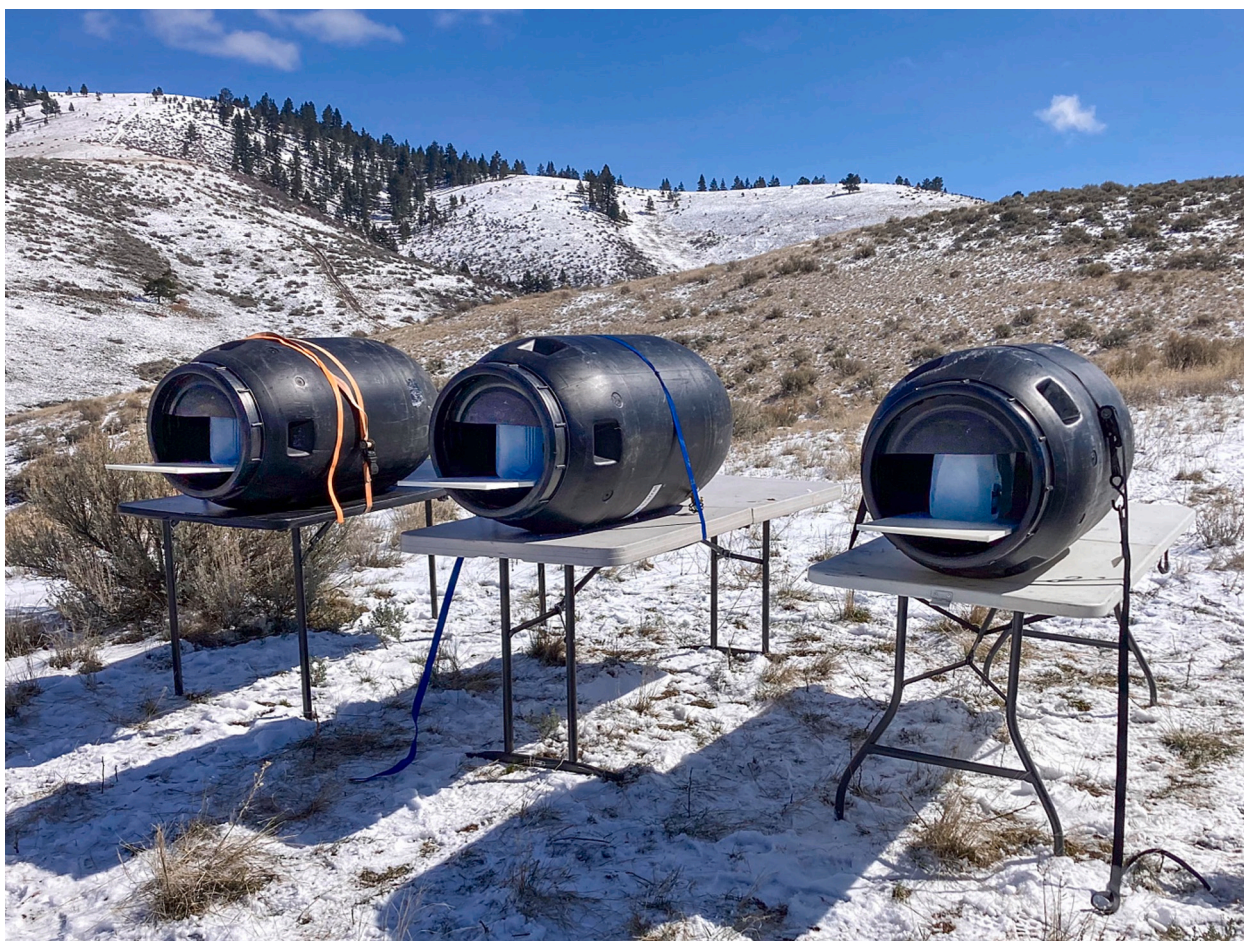
Fig. 1. We constructed three water traps to capture rifle bullets. Each trap held a row of six 3.8-L water containers.
