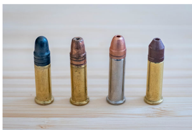
FIGURE 1 Photo of the 4 types of .22 long rifle ammunition used for precision testing on 2 March 2021 in western Montana, USA. The names of each ammunition from left to right are CCI Standard Velocity (lead-based), Winchester Super X (lead-based), CCI Stinger (lead-based), and CCI Copper-22 (lead-free)
