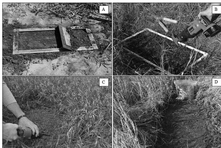
Figure 2. Soil sampling procedures to determine lead availability to ring-necked pheasants in Lyman County, South Dakota, USA, 2012–2013. A metal quadrat with associated scraper blade was used to collect 1.3 cm of surface soil for cropland and food plot samples in Study Site 1 (A). A cordless reciprocating saw fitted with a scraper blade was used to collect soil samples from grassland samples in Site 1 and all samples in Site 2 (B–D).
