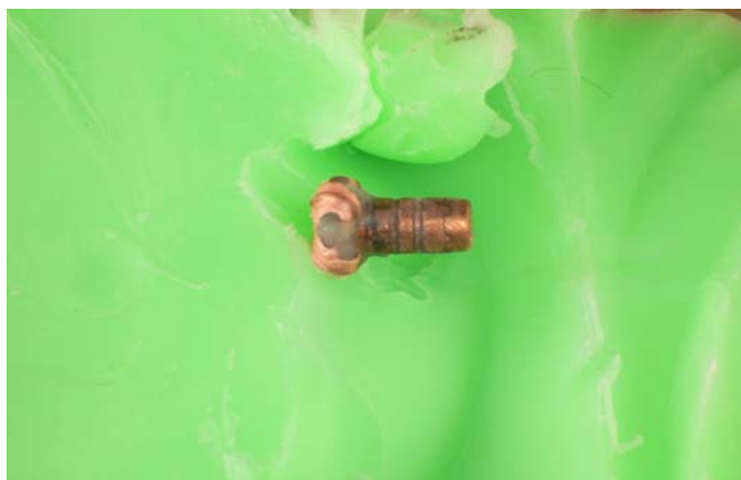
This is a close up of the bullet, 100% weight retention and a perfect mushroom.
