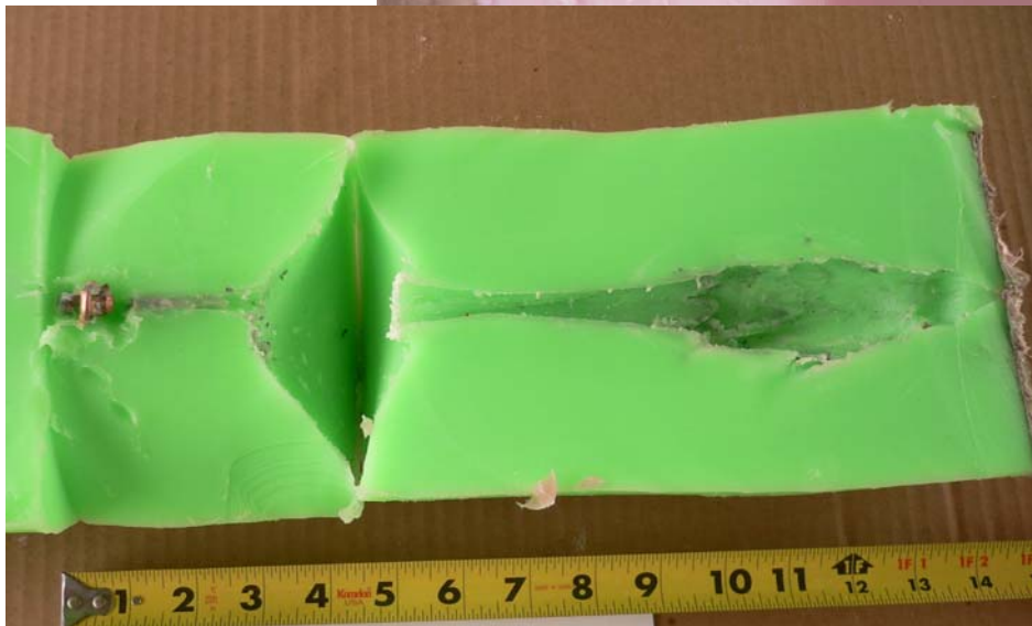
150 gr Nosler Ballistic Tip in 308 Win. The dark shading in the cavity is lead particles and lead dust.
