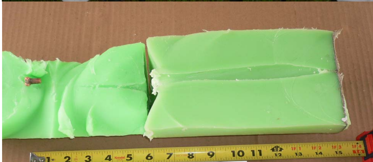
This is a 308 Win caliber Barnes 150 gr TSX bullet that penetrated 15" of the media.
