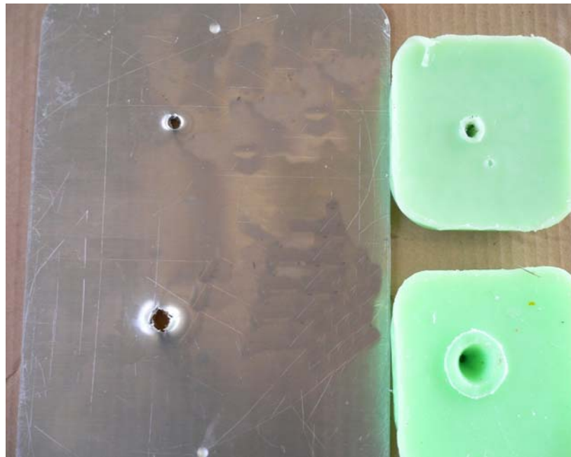
270 Winchester, 130 gr @ 1800 fps (reduced load) 1 1/2" media + 1/8" aluminum
