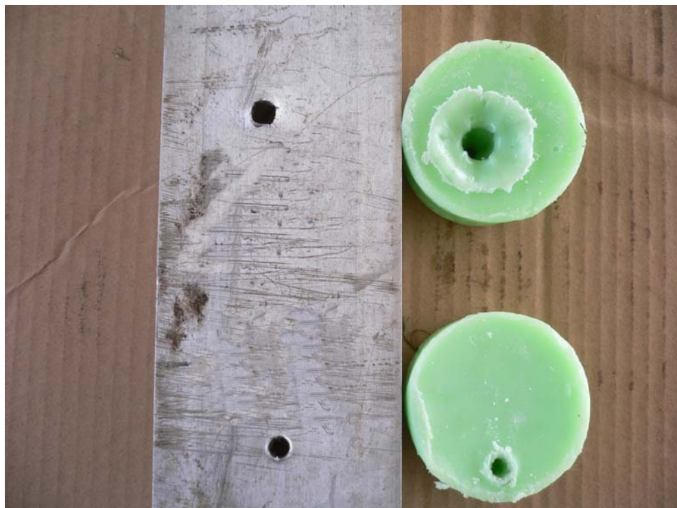
270 Winchester, 130 gr @ 1,800 fps (reduced load) 1 1/2" media + 1/4" aluminum
