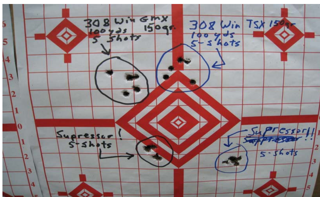
308 Win TSX and GMX 5-shot groups, with & without the suppressor, at 100 yards!!
